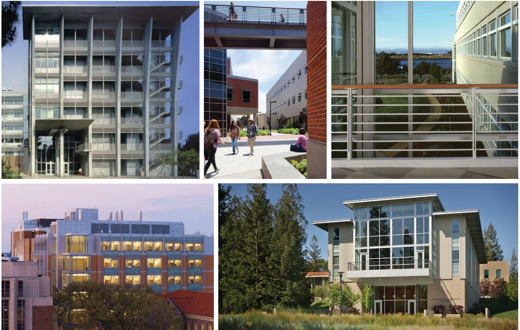
Outdoor circulation can provide depth to the building facade (top left), and architectural interest when connecting two buildings (top center). Semi-enclosed spaces can provide smaller gathering spaces on upper floors of buildings, and can take advantage of views (top right). Material transitions between base, middle and top can add visual interest to large lab buildings (bottom left). Clerestory windows, a large bay window, and roof overhangs “break the box” of a lab building (bottom right).
