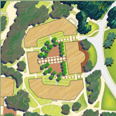
The Wellman Courtyard initiative will remove trailers from the courtyard and realize the Howard vision of a garden court following the original Tuscan plant palette. This initiative also intends to provide a site for the campus outdoor sculpture collection.
